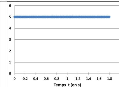
$$\text{Equation : } v_x(t) = v_0 \cos \alpha$$
